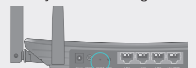
RESET Button: Press & Hold for 2 Seconds
